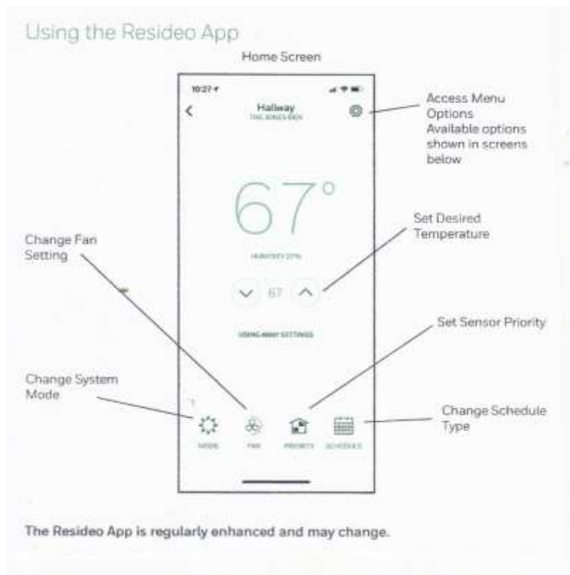
Figure 9-Rectory HVAC Phone App Control
